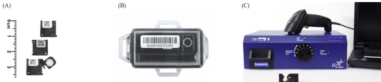
Fig. 1. Equipment used for dose measurement: Optically stimulated luminescence dosimeter (OSLD) nanoDot type (A), Inlight type (B), and Microstar reader (C).
